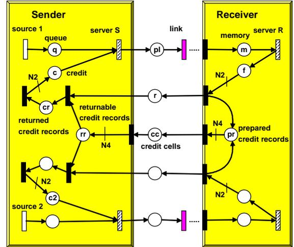
Figure 2: Petri-Net model of the flow control
