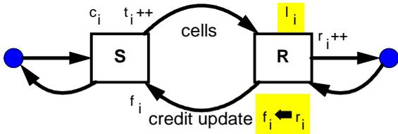
Figure 1: The basic credit flow control loop
