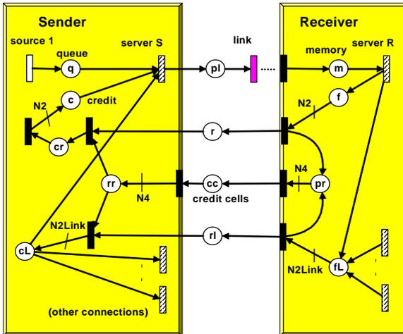
**Fig. 7: Buffer sharing by using link flow control**
