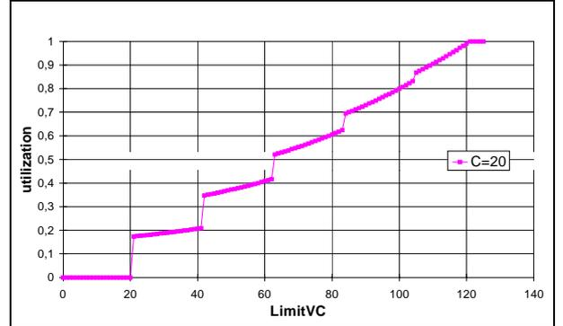
Figure 5: quantization effect of credit feedback
