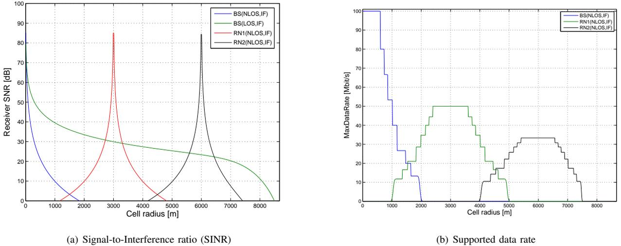
Fig. 3. Analytical analysis of a coverage extension scenario with one BS and two relays. A line-of-sight link or antennas with gain between BS and relays is assumed. An interferer is positioned at 9000m.
