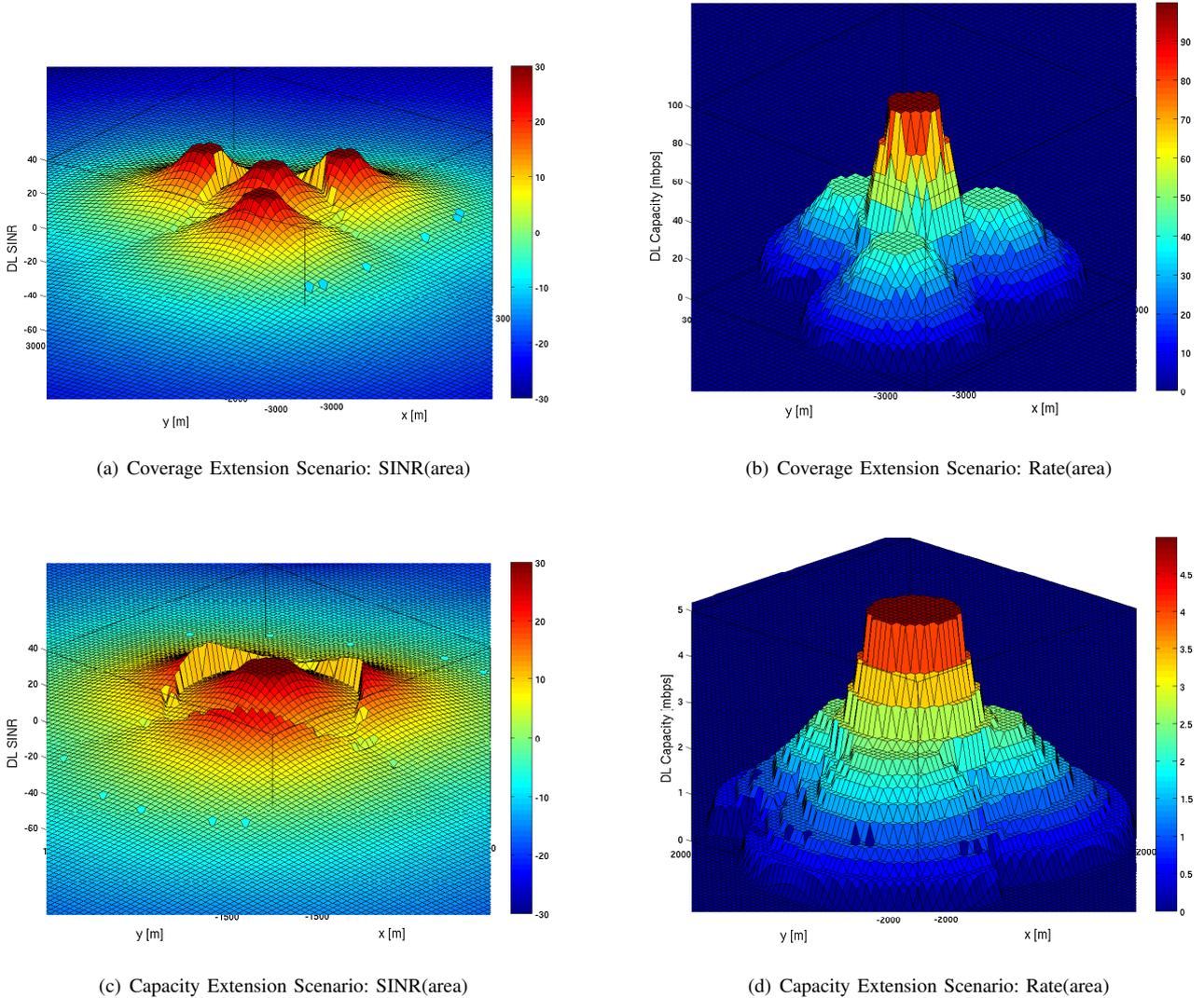
Fig. 4. Results for the two basic relaying scenarios. Values are for 3GPP-LTE, but the principles are the same for other technologies. In the graphs, a DL capacity close to  $100\text{Mbit/s}$  in the center is achieved in both scenarios. See [8] for similar WiMAX related results.
