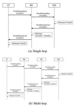
Fig. 6: Flow release signalling
