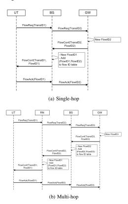
Fig. 5: Flow establishment signalling
